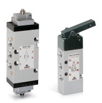
The particular mechanical device allows these end-stroke valves to operate with very low actuating forces. Series 3 has been designed with a mechanical lever device which works in negative pressure. To increase sensitivity it is possible to add to the lever a steel extension with Ø 3 mm.
