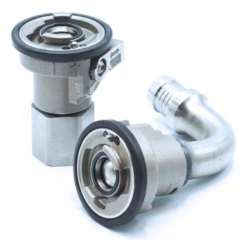
Danfoss Hansen's FD83 coupling is designed for fluid transfer and electronics cooling applications where full flow, fluid compatibility and safety are essential. The FD83 identical halves include two interlock features to eliminate spills and ensure maximum safety. Valves cannot be opened until the coupling halves are mated and coupling halves cannot be disconnected until both halves are closed.
