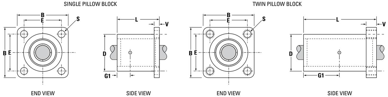
Flanged Single Pillow Blocks with Self-Aligning Bearings
