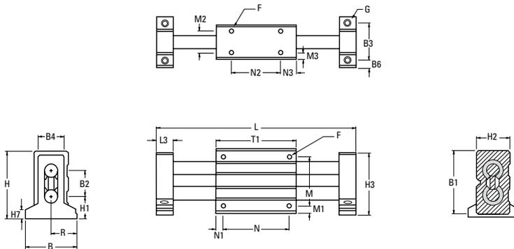
Twin Shaft Web Linear Guide with Universal Carriage (Horizontal Configuration)
