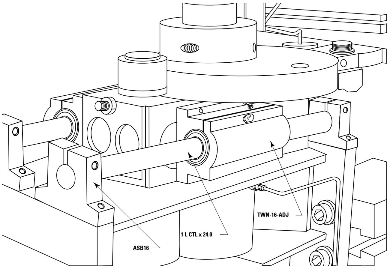
Inch – Precision Steel Ball Bushing Bearings
