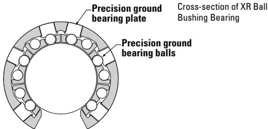
Cross-section of XR Ball Bushing Bearing
