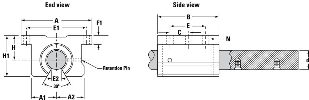
Rigid steel housing and high performance Super Smart Ball Bushing Bearing combine to reduce deflection and cost up to 66%.
