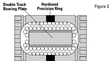
The third component is the rolling element. Each Super Smart Ball Bushing Bearing features precision ground balls manufactured to the highest quality standards for roundness and sphericity. The result is maximum load capacity, travel life and performance.
