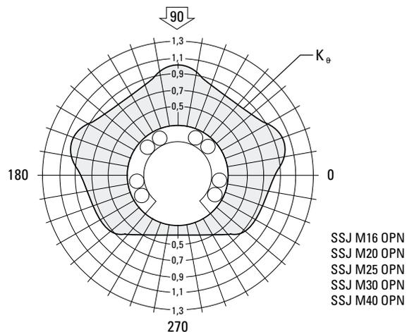
For Super Smart Ball Bushing Bearings mounted in a housing and with LinearRace shafts, h6 tolerances
