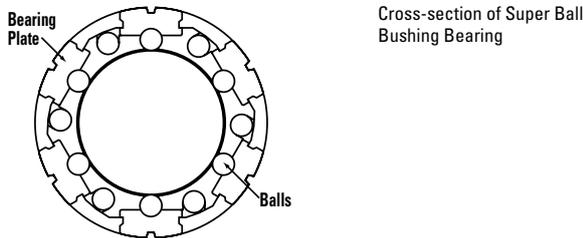
Cross-section of Super Ball Bushing Bearing
