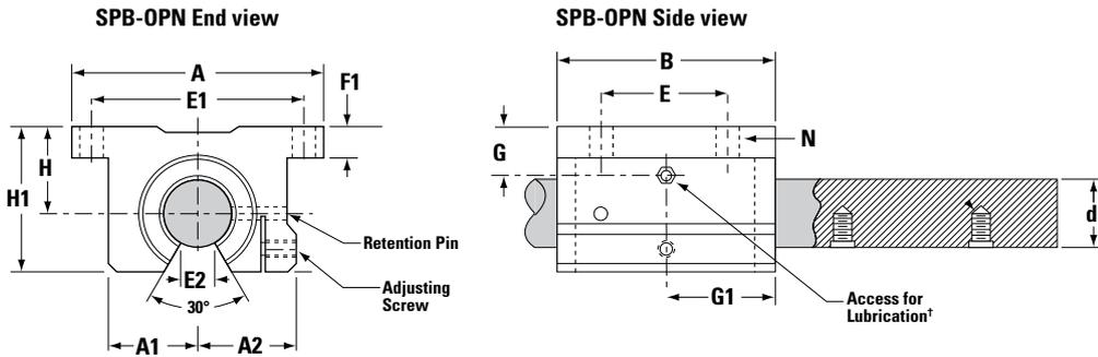
† Size .500 has oil lubricant fitting. Sizes .625 and above have 1/4-28 access for lubrication.
