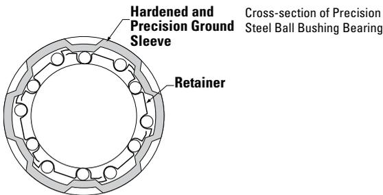
Cross-section of Precision Steel Ball Bushing Bearing
