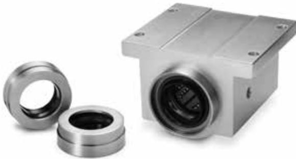
Thomson Lube for Life pillow blocks provide continuous bearing lubrication and enhanced protection for a broad range of applications. Self-lubricating cartridges are pressed into each end of the pillow block housing, and the linear bearing is lubricated initially with EP2 grease. The Lube for Life polymer is under constant pressure against the 60 Case shafting, ensuring a film of lubricant between the ball bearings and the inner race.
