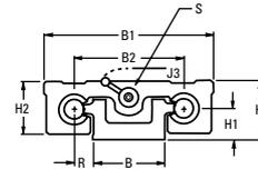
**Dual Shaft Rail Fully Supported System with Integrated Carriage (Long Style)** (Dimensions in inches)
