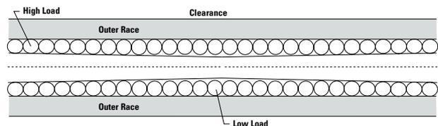
taper increases, balls go in and out of preload causing premature wear and reduction in travel life.
