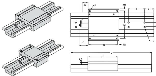
Dual Shaft Rail Supported Cross-Section
