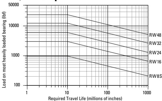
(Lines indicate limiting load for given RoundWay bearing)
