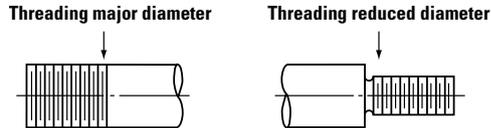
Standard threads are either Unified National Coarse or Unified National Fine, Class 2-A fit. Shafts will be annealed and soft around the circumference of threaded areas within the case.
