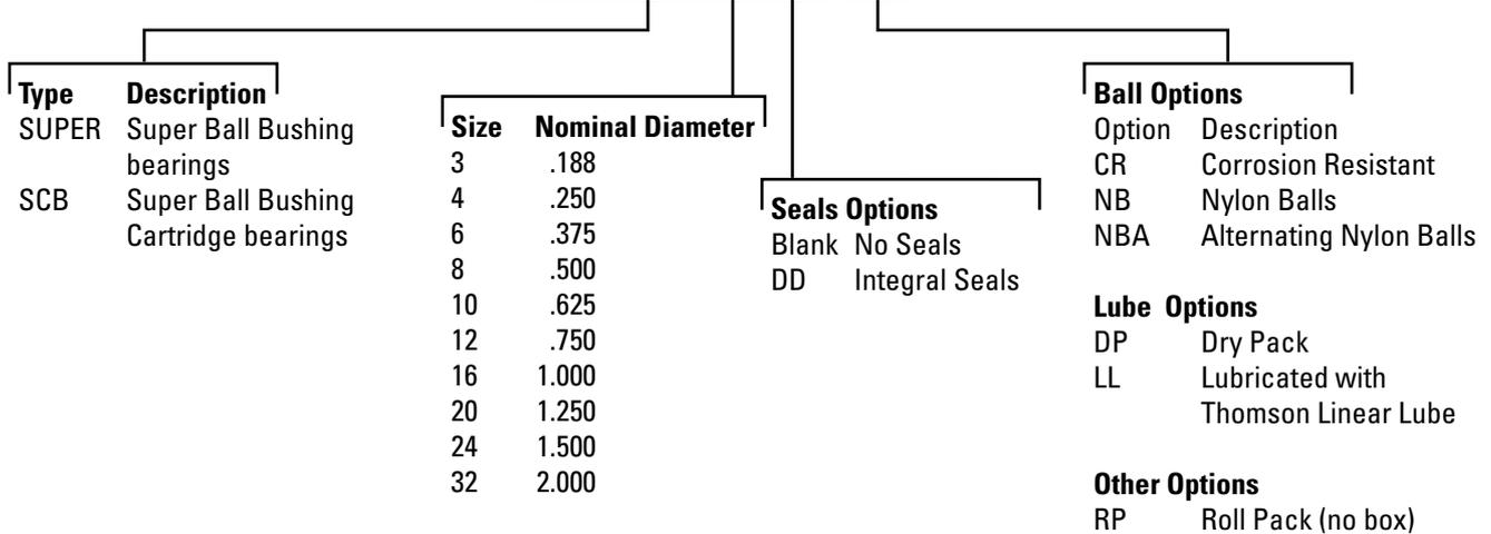
**Super Ball Bushing Pillow Blocks (Closed Type) for End Supported Applications**
