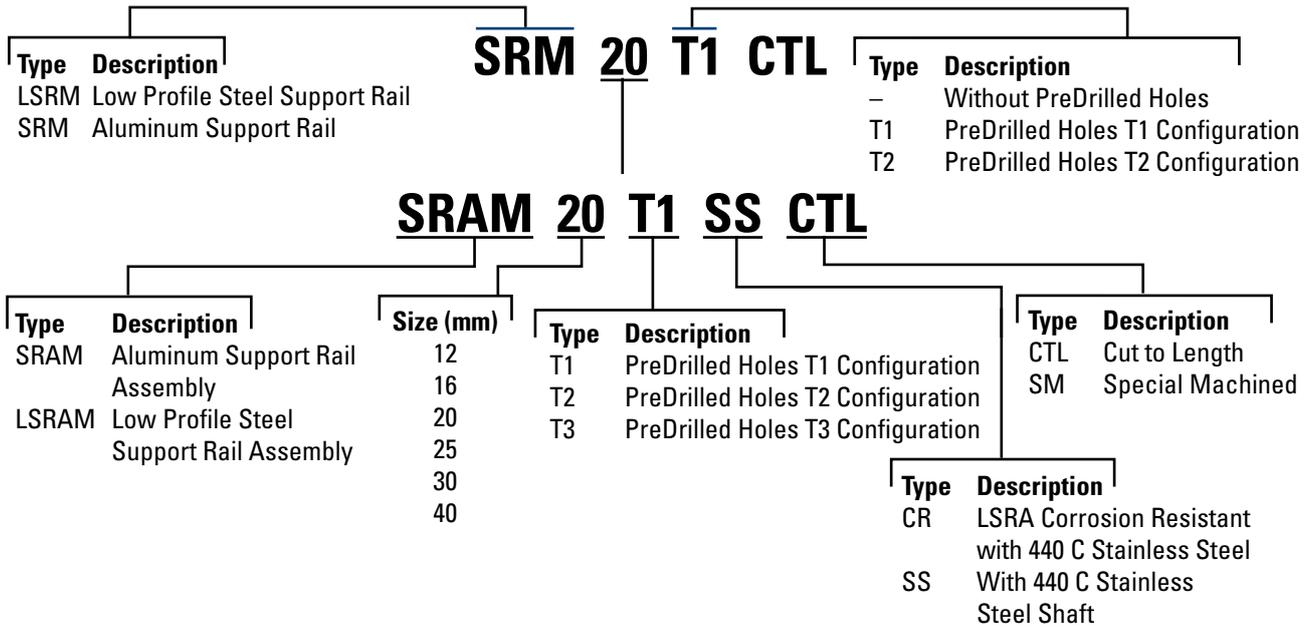
**Shaft Rail Supports Type SRM, SRM-T1 & SRM-T2**
