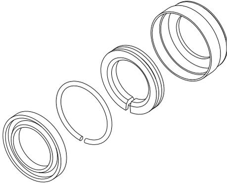
Lube for Life modification kits provide continuous bearing lubrication and enhanced protection for a broad range of applications. The Lube for Life attachments consist of a section of oil saturated polymer actively compressed by a contact spring, inside a standard Pillow Block seal. Mod Kits are for use with non self-lubricating Super and Super Smart Ball Bushing bearing Pillow Blocks. Each Mod Kit includes 2 Lube-for-Life cartridges and assembly instructions.
