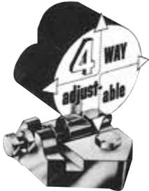
Designed for use with Roundway bearings. Two or more can be used to provide intermittent support and adjustment along the length of the shaft. Unlike shaft support rails, Waymount supports do not permit longitudinal passage of open-type Ball Bushing bearings. When it is necessary to travel over Waymount supports, Roundway bearings should be used. Open-type Ball Bushing bearings can be used only if side loads are light and an adapter block is used (consult factory for recommendation).
