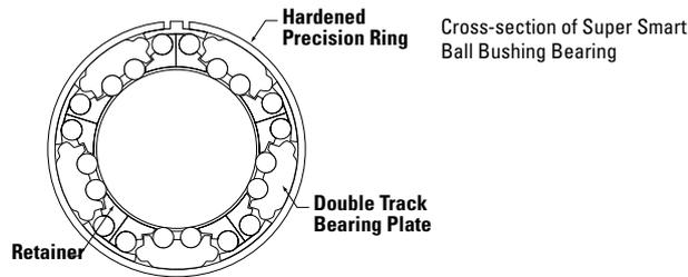
Cross-section of Super Smart Ball Bushing Bearing
