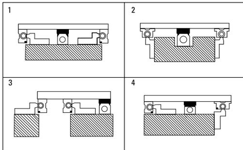
Pillow blocks shown are the standard SSUPBO or SPB-OPN style. To order System 1DA with standard pillow blocks, order the Side Mounted Shaft Rail Assembly (SSRA) and the SSUPBO or SPB-OPN separately.
