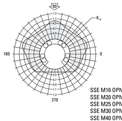
For Super Smart Ball Bushing Bearings mounted in a housing and with LinearRace shafts, h6 tolerance
