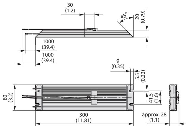
**Dimensional drawing, braking resistor, A3**
