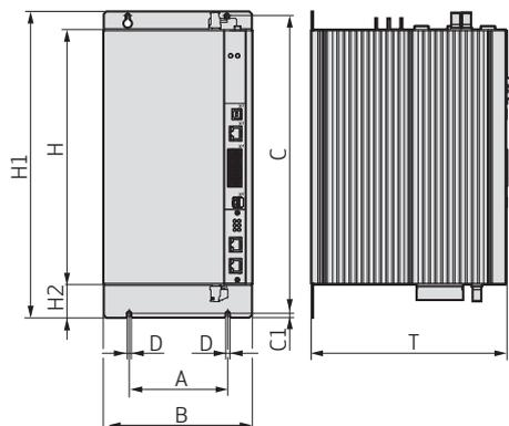
Installation drawing, Liquid-cooled
