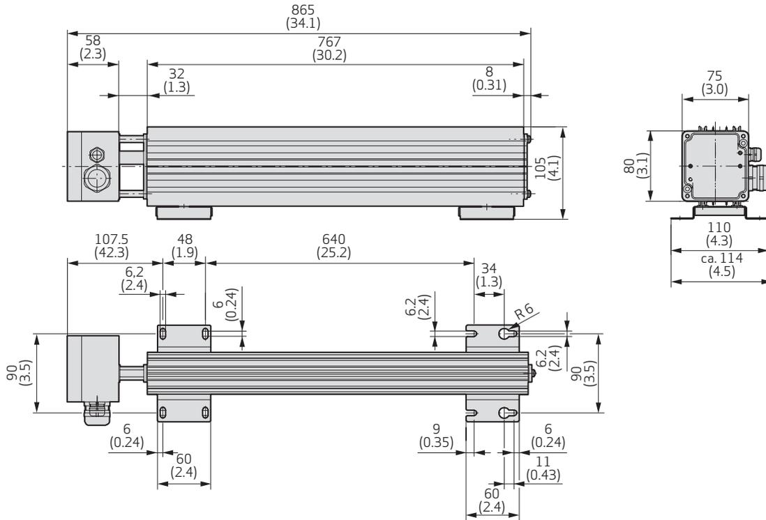
**Dimensional drawing, braking resistor, A5**
