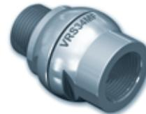
The VRS Series Vacuum Rotary Connection, with its robust and lightweight design, provides an in line rotary connection for vacuum supplies. Its continuous rotation system avoids coiling of the hose and eliminates force constraints when used with collaborative robots.
