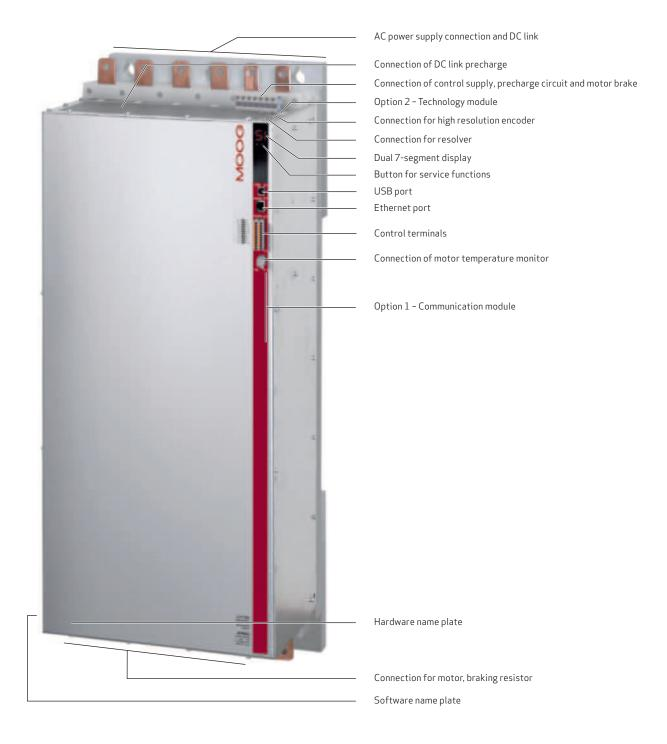
The maximum permissible servo drive rated current and peak current are dependent on the mains voltage, the motor cable length, the power stage switching frequency and the ambient temperature. If the conditions change, the maximum permissible current capacity of the servo drives also changes.
