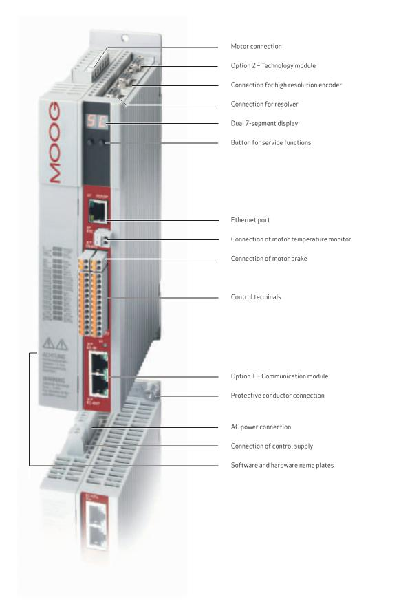
The rated current of the Single-Axis Compact, overcurrent (200 % rated current) and the maximum peak current (300 % rated current) are dependent on the mains voltage, the motor cable length, the power stage switching frequency and the ambient temperature. If the conditions change, the maximum permissible current capacity of the servo drives also changes.
