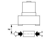
(Note) O type gripping power decreases approximately 20 to 30% in the closed direction compared to double acting. C type gripping power decreases approximately 10 to 20% in the open direction compared to the double acting. When making a selection, read the precautions for design and selection on page 1872.
