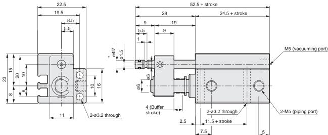
\* Recommended inner diameter tolerance of the mating side's socket: H8
