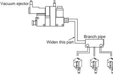
Perform piping with a sufficient effective crosssectional area. For the vacuum piping side, select a piping with sufficient effective cross-sectional area to allow the flow of the max. suction flow rate to the ejector.
