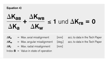
Diagram 1: Miasalignment Chart for Couplings with one Disc Pack (Single-Jointed Design)
