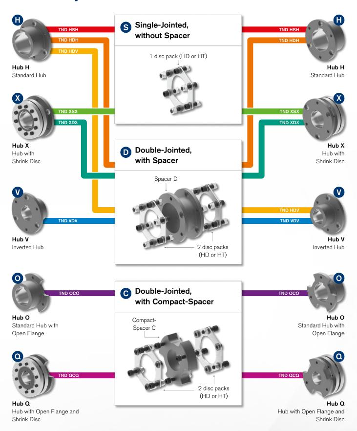
The smart modular system of the RINGFEDER® TND series guarantees users maximum flexibility and customizability to fulfil the specific requirements of their individual drive task. By virtue of the various combination possibilities and multiple extension options, further coupling types are realizable in addition to those depicted
